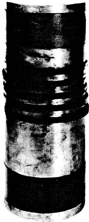
Figure 4. A nonlube piston removed from an engine after a test run. FXA piston, bottom view, 175 hr.
